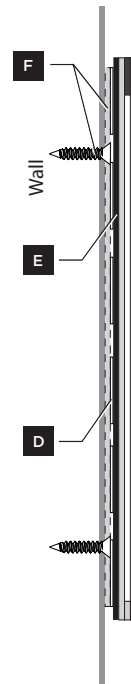
MOUNTING (VHB tape and mechanical fasteners)
