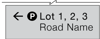
PNL.2- Variation 1/2" = 1'-0" Multiple lots may be directed to if they are located on the same street.
