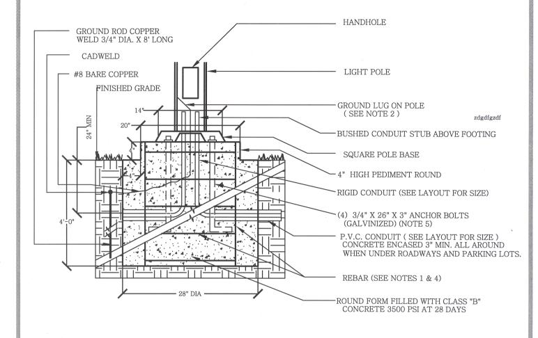
NOTES: SEE PLAN FOR LOCATIONS OF EXISTING FIXTURES TO REMAIN. PROVIDE GROUND ROD 3/4" X 8' AT EVERY OTHER POLE AND CONNECT TO GROUND LUGS IN POLE BASE & TO GROUND WIRE.
